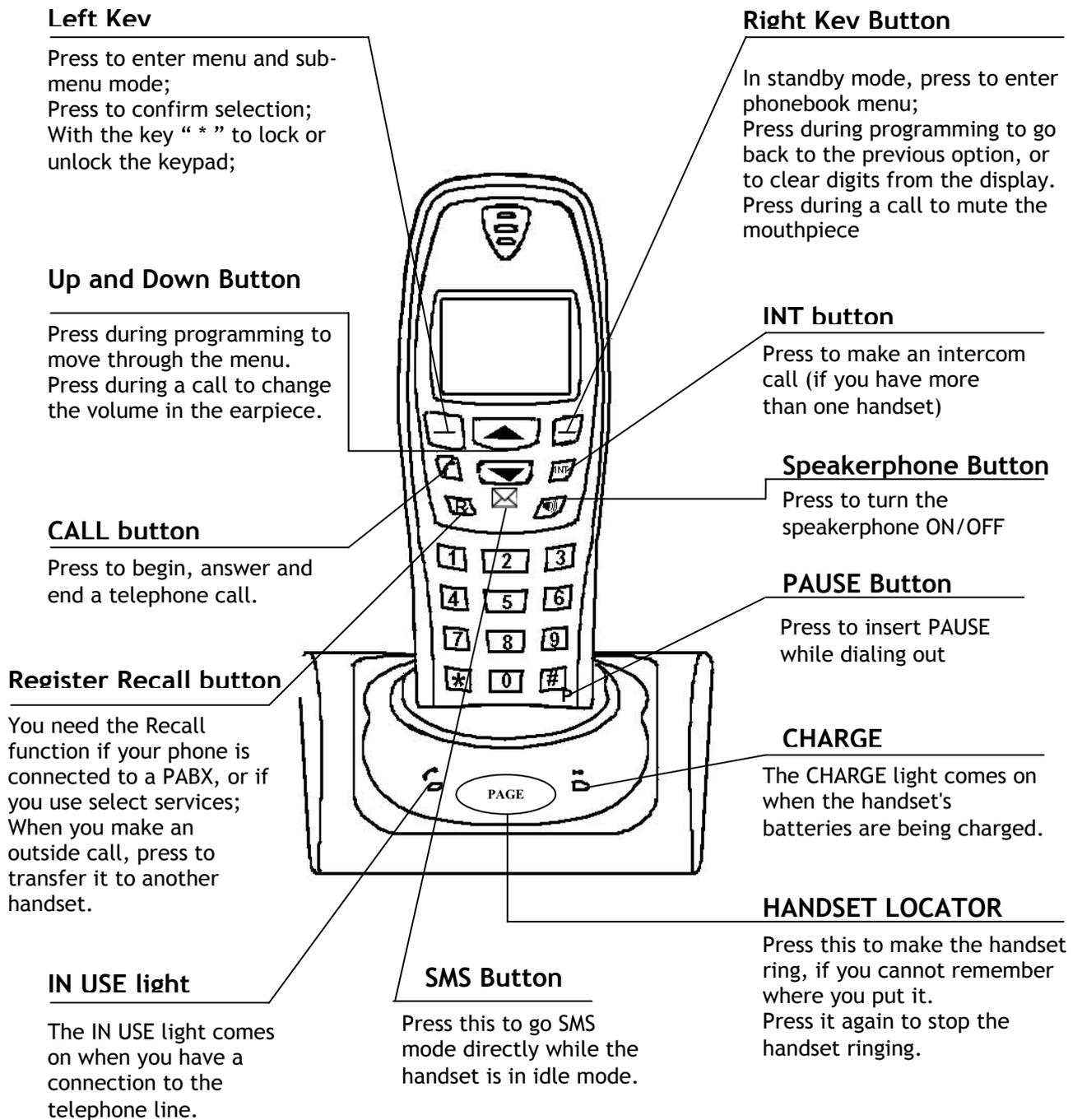
Before you can use the handset to make calls for the first time, you will need to fit and fully charge the battery for 15 hours.
